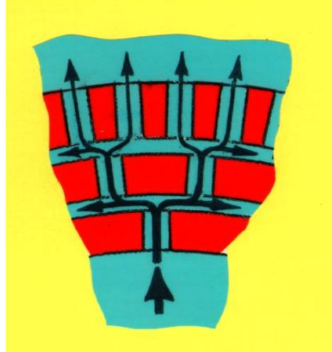
Fig 5. Flow path through a cascade trim
