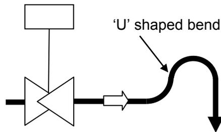
Fig 3. Installation of a Downstream Bend
