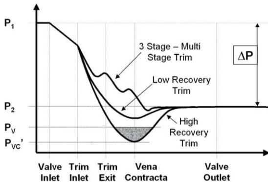
Fig 4. Treatment of Cavitation Using the Valve Trim
