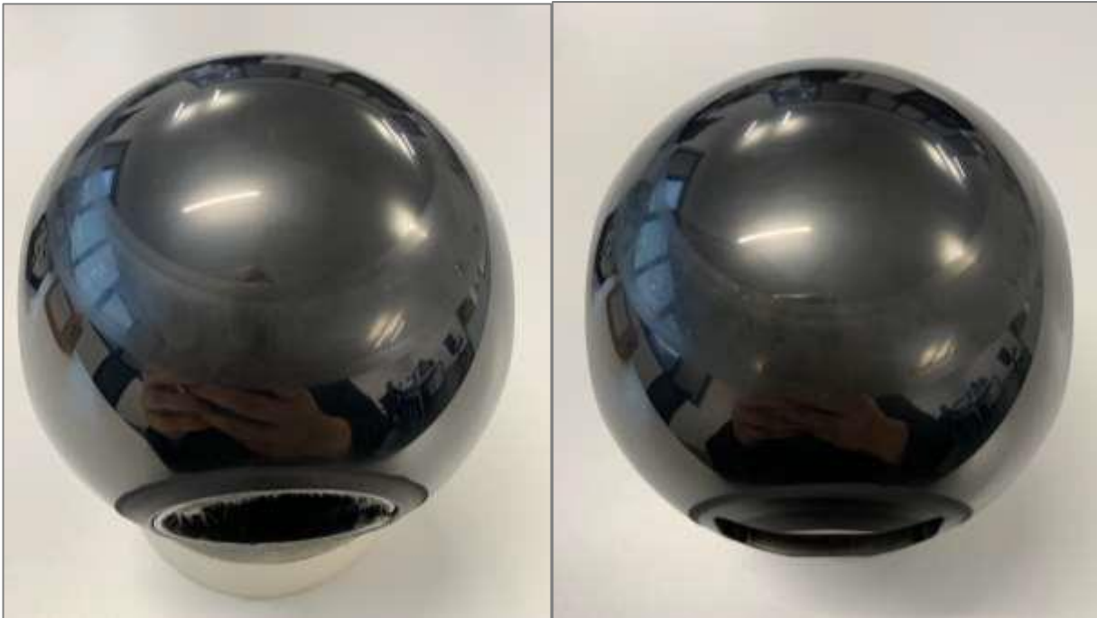
Figur 5: Ball side A (on the left) and side B (on the right) after the qualification tests for FC actuated valves. No relevant damage appears on the ball surface as confirmed by leakage rate results, which remain under Rate B.
