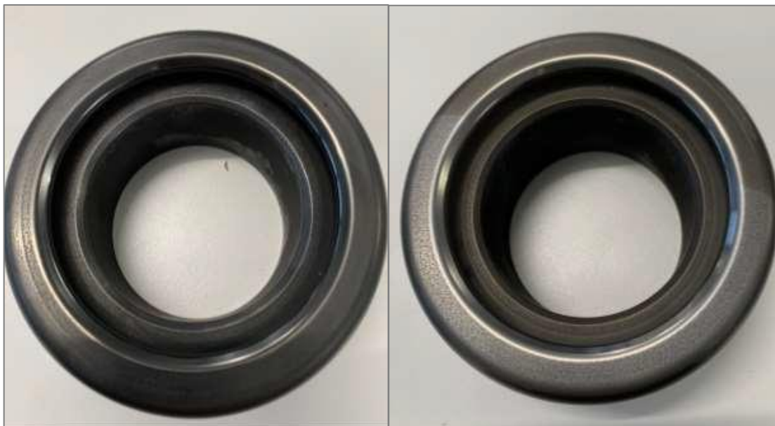
Figur 5: Ball side A (on the left) and side B (on the right) after the qualification tests for FC actuated valves. No relevant damage appears on the ball surface as confirmed by leakage rate results, which remain under Rate B.
