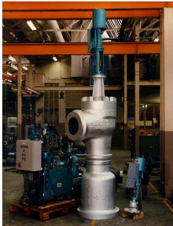
Turbine Bypass Valve & Spraywater Control Valve Fitted at Didcot B Power Station. The Valve is Mounted on its Side
