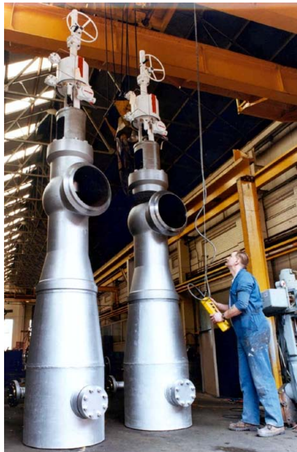
Turbine Bypass Valves for Lost Pines Power Station
